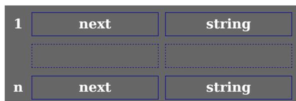
The hash value (integer calculated from string) point to a slot and the string is compared with the stored string. When the string is different, the next field points to a different slot (outside the hash range in the same table) and again the string is checked. When there is no next value set (zero), the index is used to determine what to do.
