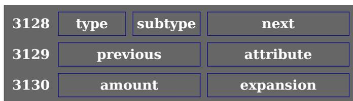
So here we take a slice of three memory words from the node array starting at index 3128. We mention this detail because sometimes (when tracing) you see these numbers. This doesn't mean that at that point we had 3128 nodes, because the next node taken from this pool will have number 3131. The numbers are indices!
